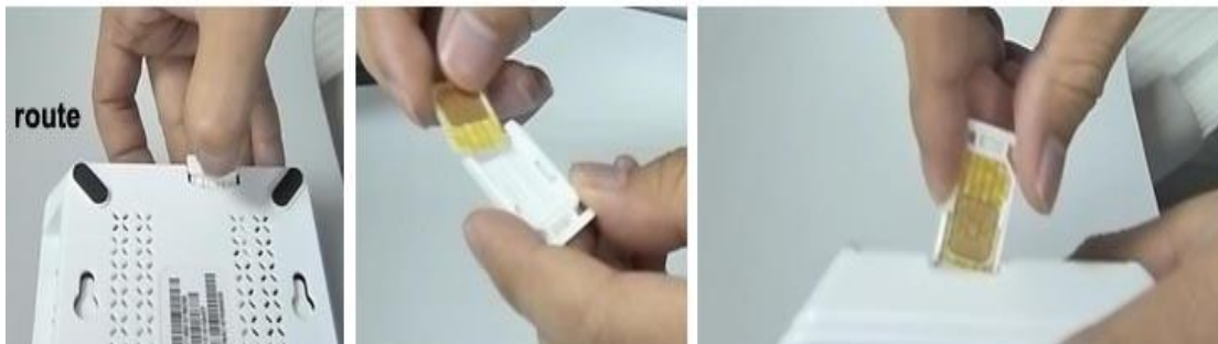
Inserting 3G SIM card steps
