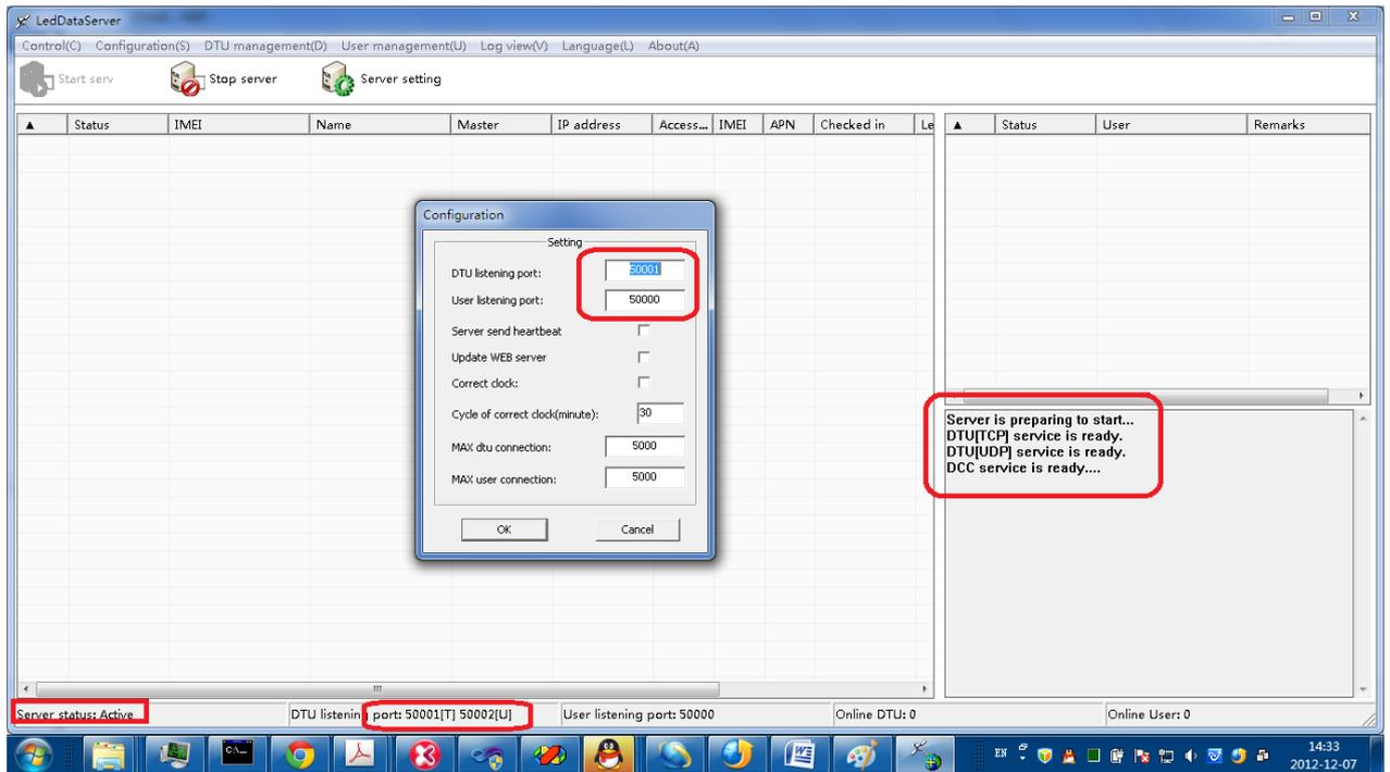
Step3, set port forwarding in Router, Forwarding port 50000-50002 to server, IP address is the server's IP in LAN.
